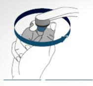
2. Install your new faucet cap with aerator - Align the threads on the inside of the faucet arm with the exterior threads of the new cap. Turn the faucet cap in a clockwise (right) direction and tighten fully.
