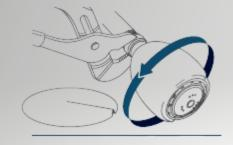
**1.** Remove existing showerhead - Grip the base of your showerhead and turn counter-clockwise (left) to loosen. Use pliers if necessary.
