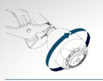
**2.** Install your new, energy-efficient showerhead - Twist your new showerhead onto the threaded area of the shower arm in a clockwise direction (right)
