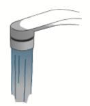
**3.** Test your new aerator - While the water is flowing, look closely for any leaks at the threads. If you notice a leak or spray, tighten.
